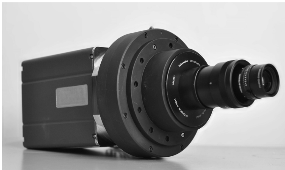
Fig. 3. 16-MegaPixel-CCD Camera (Peregrine 486) equipped with a lens of the type Schneider Kreuznach Macro Symmar 5.6/120.
